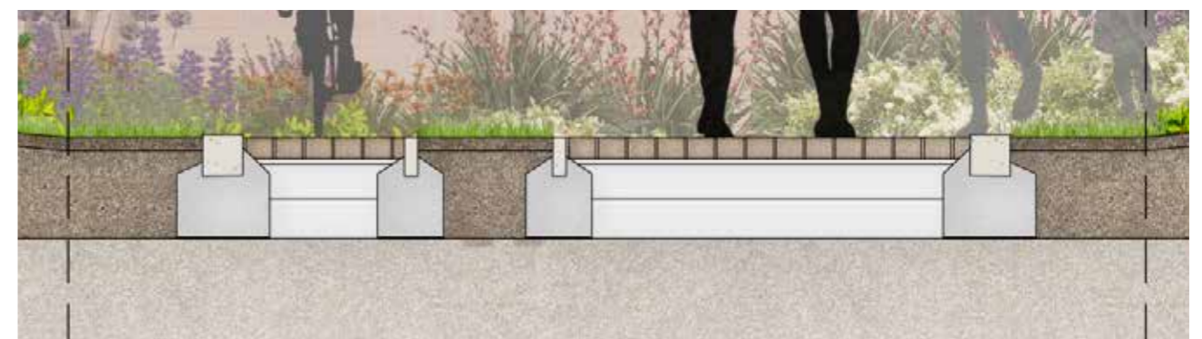
Reinforced grass 500mm | Cycle lane 1000mm | Reinforced grass 500mm | Footpath 1500mm | Reinforced grass 500mm
